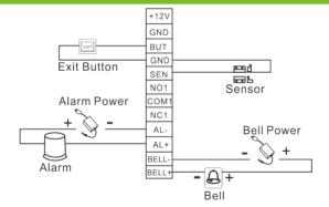
Only devices with an alarm consuming  $\leq$  12V DC can be connected.
