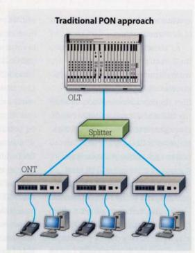
In contrast to structured cabling's "any-to-all" configuration capability, a traditional passive optical network directly interconnects the OLT. splitters and ONT via one-strand singlemode connections—a setup that has several implications.
