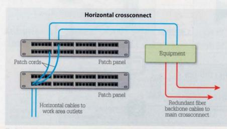
Horizontal crossconnects are a hallmark advantage of the structured cabling approach. Using patch panels, horizontal crossconnects facilitate a flexible "anyto-all" configuration through which any equipment port can be connected to any work-area outlet.
