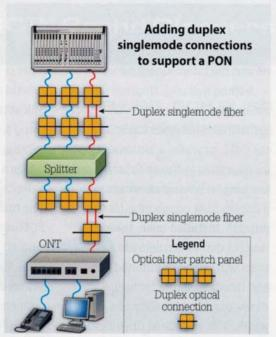
An initial step in supporting a PON with structured cabling is to replace the direct onefiber singlemode connection between OLT and splitter with a main crossconnect that supports a duplex singlemode fiber backbone connection to each outlet.
