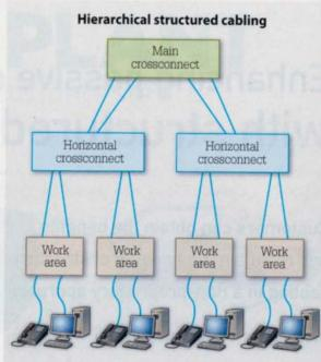
cabling added complexity and cost. In response, industry standards organizations developed and now recommend a hierarchical structured cabling infrastructure for connecting multiple network devices and supporting multiple applications, as shown in the above figure. This industry standards-based structured cabling approach enables interoperability between equipment and cabling vendors.
