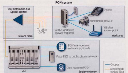
In a passive optical network, the singlemode optical fiber that connects to each optical network terminal (ONT) originates from the optical line terminal (OLT). The fiber from the OLT is split into multiple fibers at optical fiber distribution hubs containing passive optical splitters. From there, the fibers connect to the ONTs.
