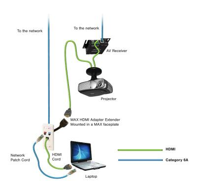
BYOD Configuration using HDMI Adapter Extender
