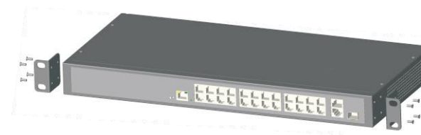
Figure 2-1 Install hangers diagram
