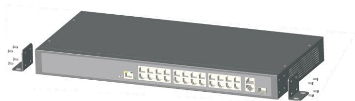
Figure 2-3 Hangers installation diagram
