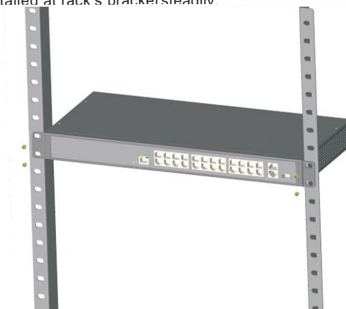
Figure 2-2 Install device to the rack
